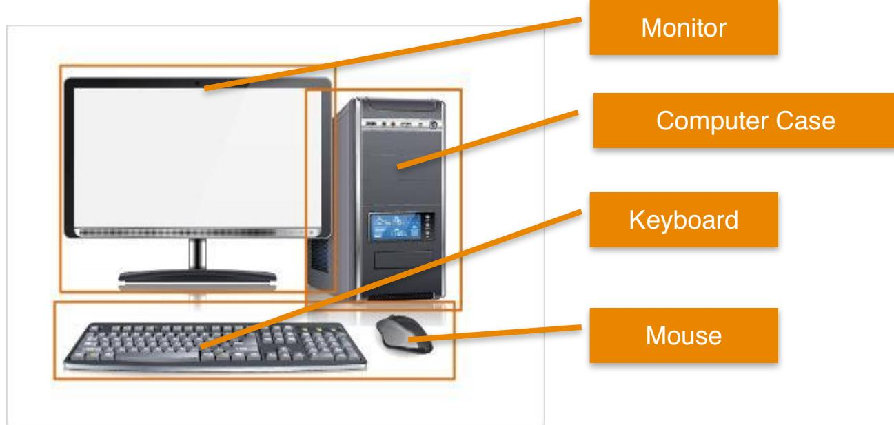
The computer case is what holds the main parts of the computer that make it work and process information.
